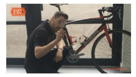
Use a 15mm spanner or an 8mm Allen key to remove your pedals.
