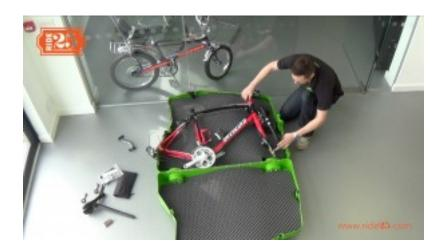
Fit the frame into the box first, and then adjust the handlebars so that they tuck in between the top tube and the fork
