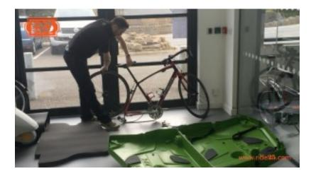
Remove your back wheel and then move onto your front wheel by loosening the wheel nut.
