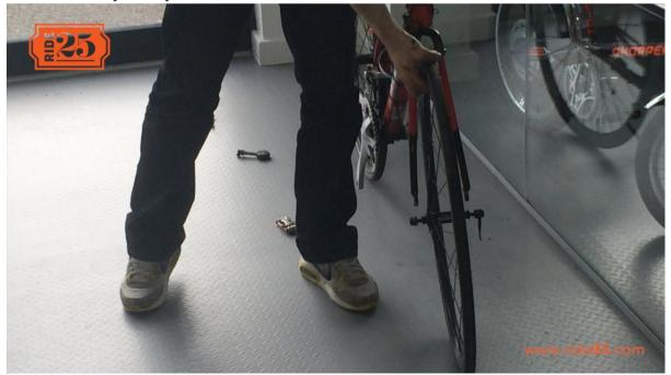
Next, get your front wheel, place the skewer through the wheel, tighten loosely and fit on to the wheel. Once it is in place, tighten the skewer (making sure it is in the middle of the wheel) and make sure the brake is on tight and in line.
